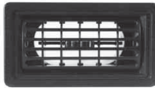
LO-25101 BLACK PLASTIC DIMENSIONS: 113mm X 65mm APERTURE: 104mm X 57mm TAKES 57mm DUCTING (can use 62mm)
